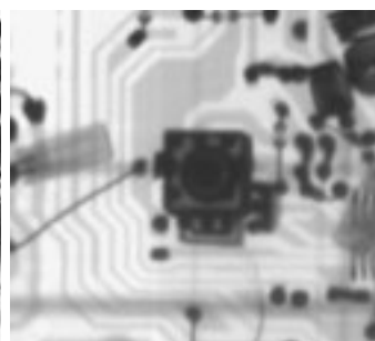
Geometric magnification with microfocus generator
